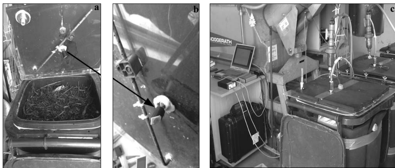
Figure 5: Positioning of the optical oxygen sensor (a, b) within the pilot bioreactor (c).
